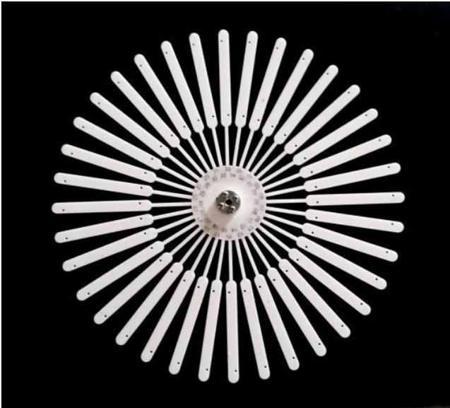
Fig. 7– The Plexiglass wheel just cut by the laser machine, with the flange for the motor shaft
