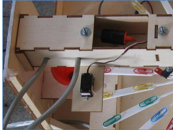
Fig. 4 – The dripper and the servo moving the gutter
