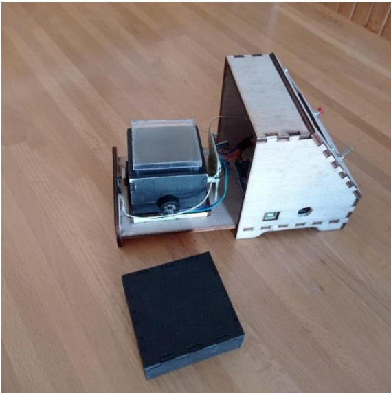
Figure 2 - The photos show the transparent cell inserted in the dark container (sample holder) with its cover. Container and cell are removable. The electronics are contained on the right side.
